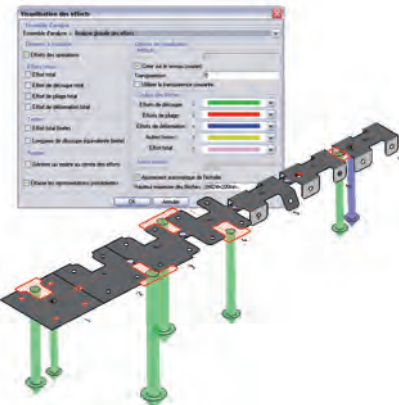
Forces analysis visualisation with TopSolid'Progress 2008.
